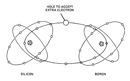
Figure 11-6. Boron-Doped Silicon.
