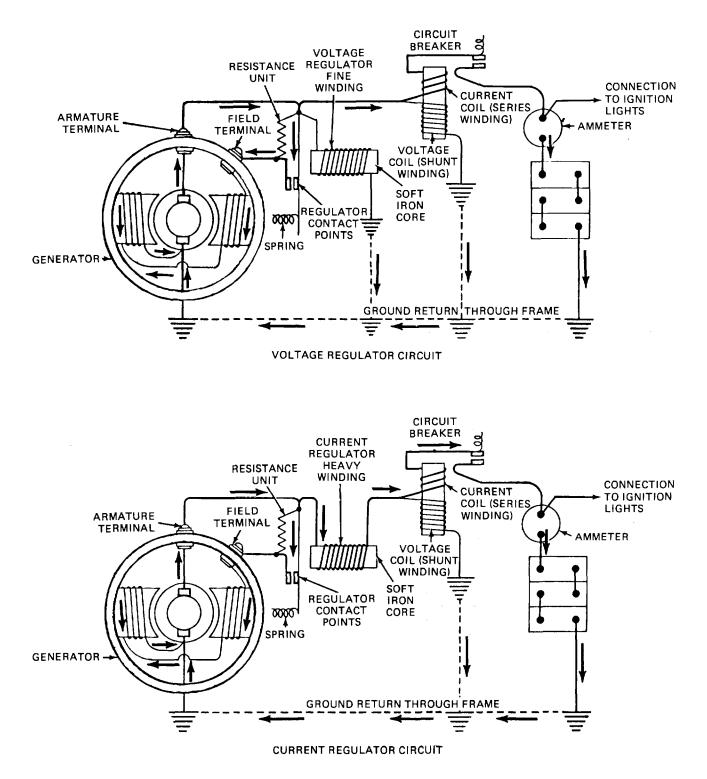
Figure 13-11. Vibrating Point Regulator Circuit.
