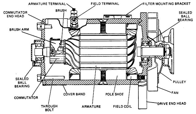
Figure 13-5. Shunt-Wound Generator.
