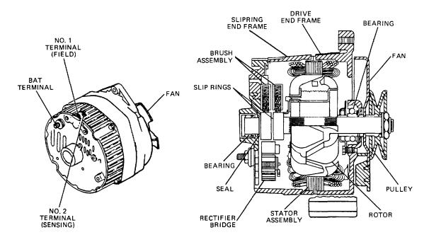
Figure 13-21. Typical Alternator.
