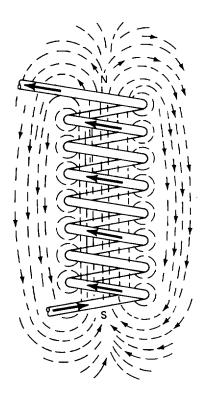
Figure 11-20. Electromagnetism in a Wire Coil.
