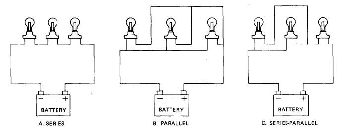
Figure 11-14. Circuit Configurations.
