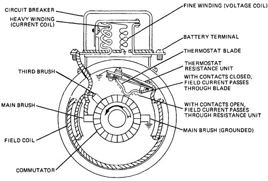
Figure 13-16. Thermostatic Control of Third-Brush Generator.
