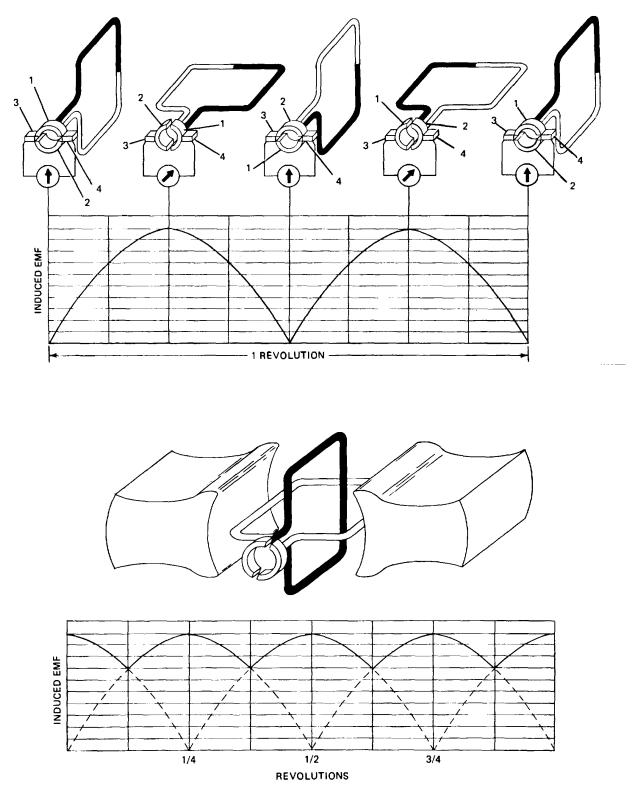
Figure 13-1. & Figure 13-2. Multiple -Loop Generator.
