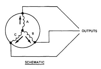
Figure 13-26. Wound-Pole Alternator.
