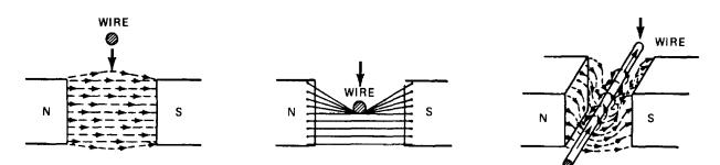
Figure 11-22. Electromagnetic Induction.
