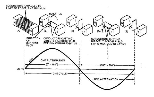
Figure 13-23. & Figure 13-24. Simple AC Generator.
