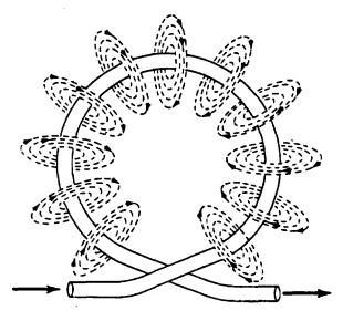
Figure 11-19. Electromagnetism in a Wire Loop.
