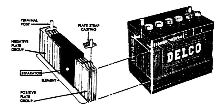
Figure 2-1. Negative and Positive Plate Group With Separators.
