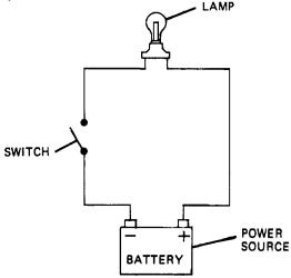
Figure 11-12. Basic Electrical Circuit.
