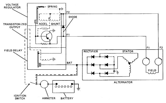
Figure 13-36. Transistorized Voltage Regulator
