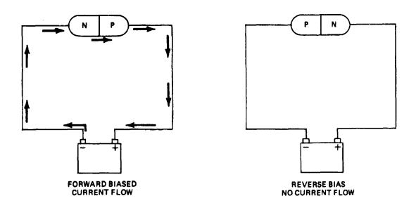
Figure 11-8. Diode Operation.
