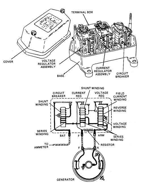
Figure 13-10. Vibrating Point Voltage Regulator.
