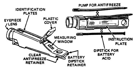
Figure 2-4. Optical/Antifreeze Tester (Duo-deck).
