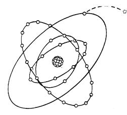
A. COPPER - CONDUCTOR (ONE FREE ELECTRON)
