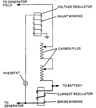
Figure 13.12. Carbon-Pile Regulator and Circuit.
