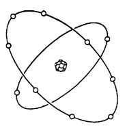
B. NEON - INSULATOR (OUTER SHELL FULL, NO FREE ELECTRONS)
