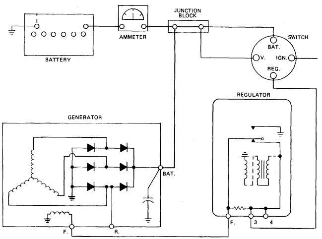
Figure 13-35. Vibrating Point Regulating Circuit
