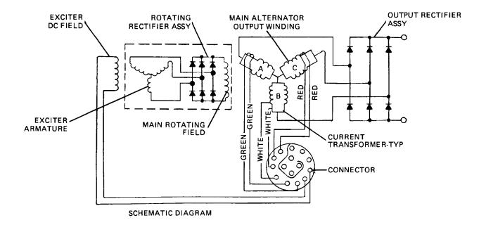
Figure 13-32. Brushless-Rotating Rectifier
