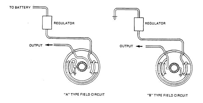
Figure 13-4. Field Winding Configurations.
