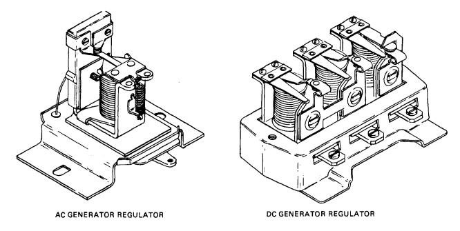
Figure 13-34. AC and DC Regulator Comparison
