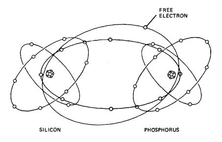
Figure 11-5. Phosphorus-Doped Silicon.
