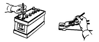
Figure 2-6. Electrolyte Sample.
