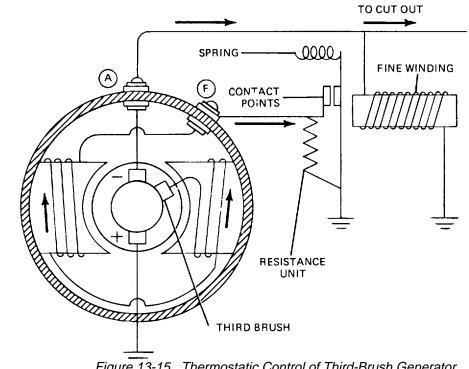
Figure 13-15. Thermostatic Control of Third-Brush Generator.
