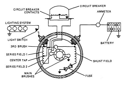
Figure 13-14. Light Switch Control of a Third-Brush Generator.
