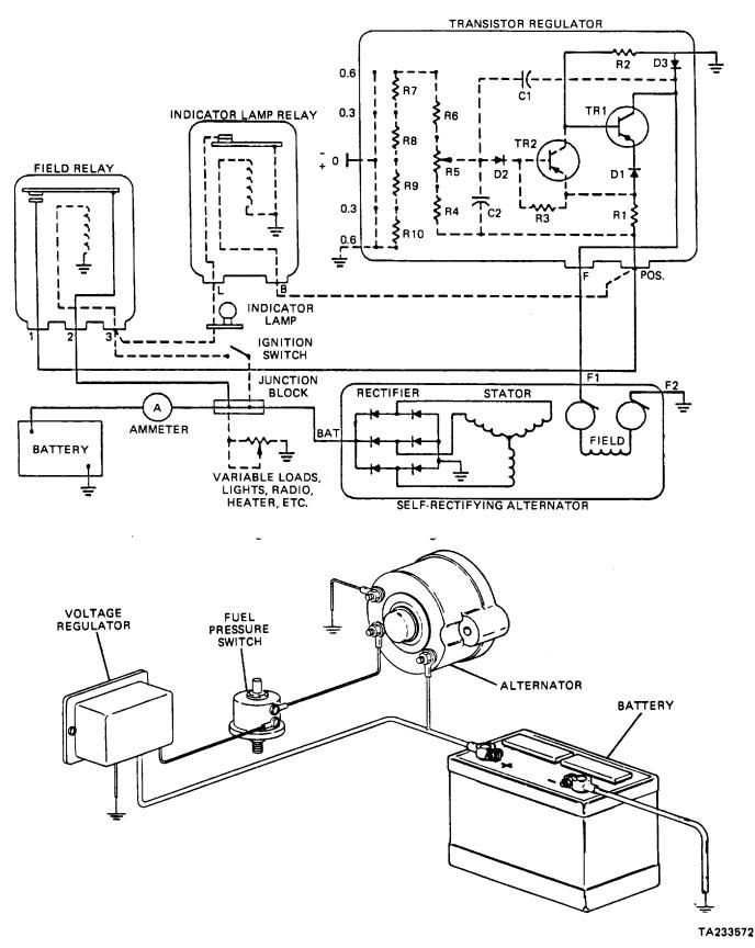
Figure 13-37. & Figure 13-38. Fuel Pressure Field Switch Circuit
