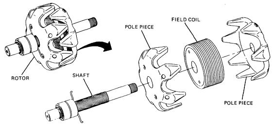
Figure 13-25. Rotor Construction.
