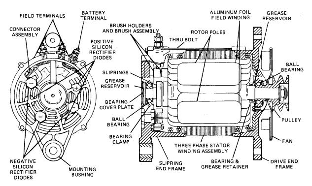
Figure 13-28. Wound-Pole Alternator.
