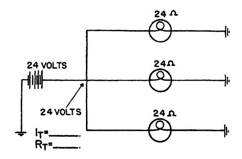
Figure 1-7. Parallel Circuits.
