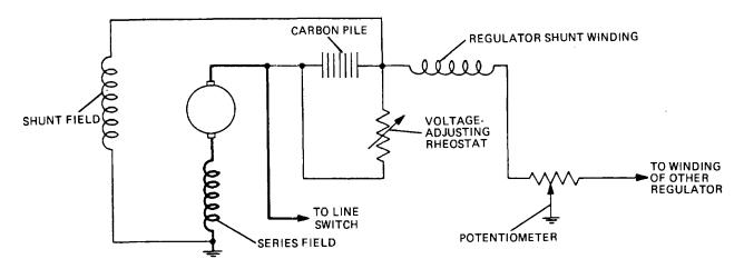
Figure 13-20. Carbon-Pile Regulation of Generators.
