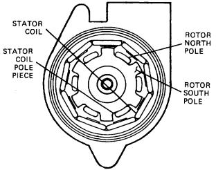
Figure 13-27. Rotor-to-Stator Relationship.
