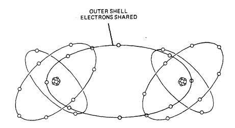
Figure 11-4. Covalent Bonding OF Silicon.
