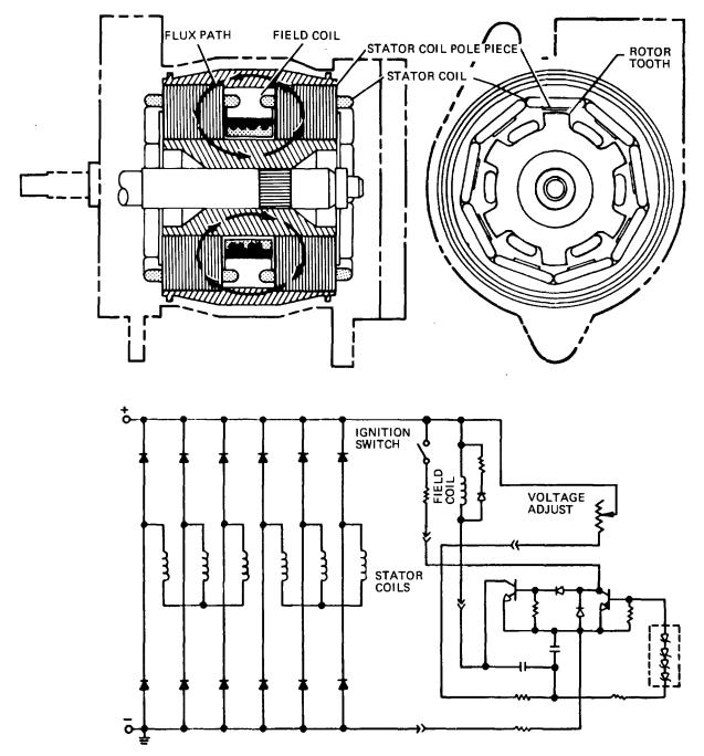
Figure 13-31. Inductor Alternator
