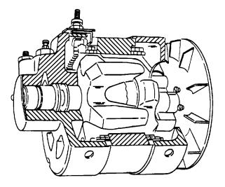
Figure 13-29. Rotor-to-Stator Relationship.
